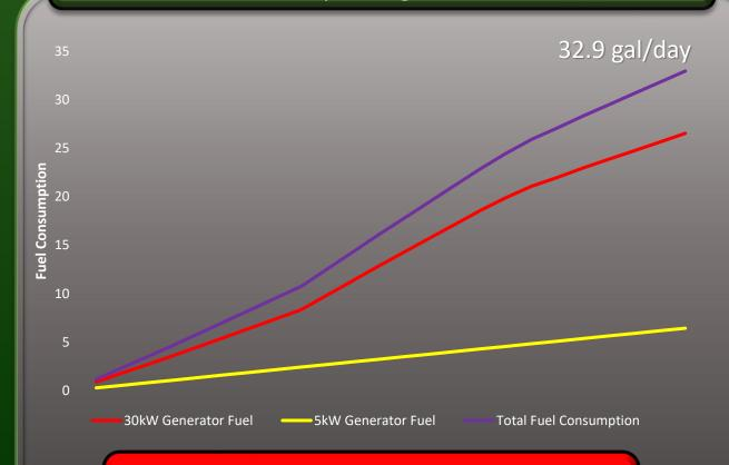
Inefficient use of generators leads to consistently higher rates of fuel consumption
