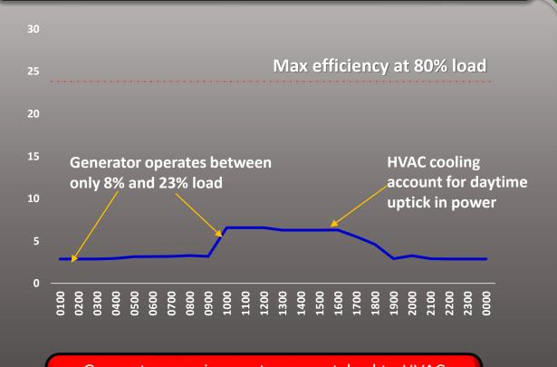
Generator requirements are matched to HVAC startup amperage, not energy profile, leading to poor generator efficiency
