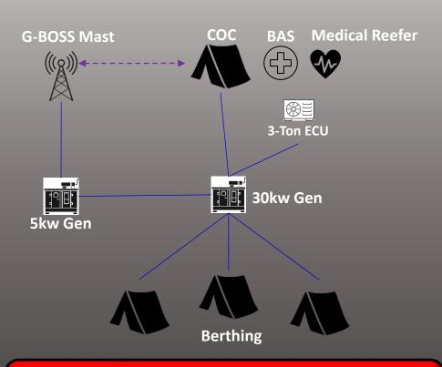
In legacy power setups, the COC and the larger Patrol Base, connect to generators based on power and <a href="mailto:peak amperage">peak amperage</a> requirements.
