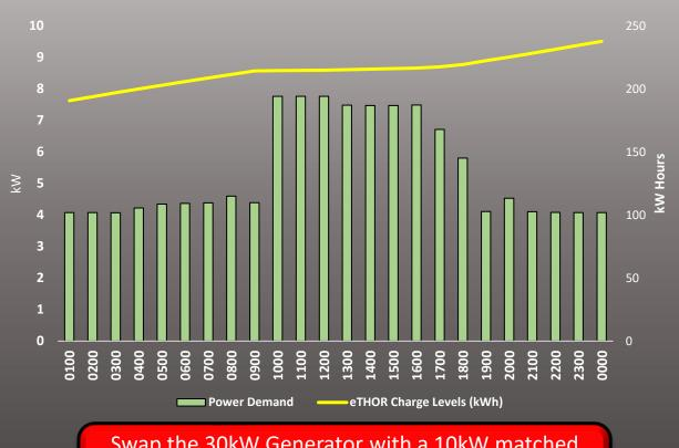
Swap the 30kW Generator with a 10kW matched and eTHOR covers all power AND amperage needs while maximizing generator efficiency
